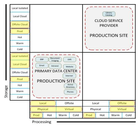
Strategy statement: Manually initiated recovery to the Hot Site which is a passive data center with a replicated SAN. SAN technology allows for near real-time replication that provides the ability to restore services to a very recent recovery point.
